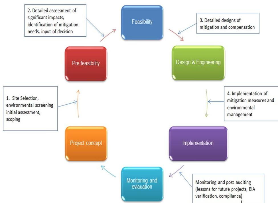
Figure 8 Environmental Management System in Project Life Cycle
